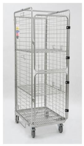
**Technical data:** the stability of construction is provided by closed profiles, nets made of steel bars, bottom with wheels (2 fixed wheels, 2 swivel wheels with brakes), the wire base is reinforced with flat iron.
