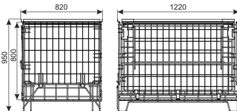
This pallet container is a full value container, making it possible to store and transport loose goods, without using euro pallets. It allows for stacking up to three containers (pallet container and the pallet) and reducing to 1/4th the warehouse floor space necessary to store the same quantity of goods. Metal feet allow the container to be lifted up by a fork-lift and also facilitate cleanliness in the warehouse.
